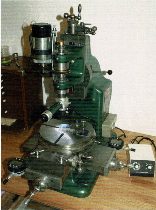
Figure 4. BCA jig borer and custom made centring microscope (based on Hemingway kit).
