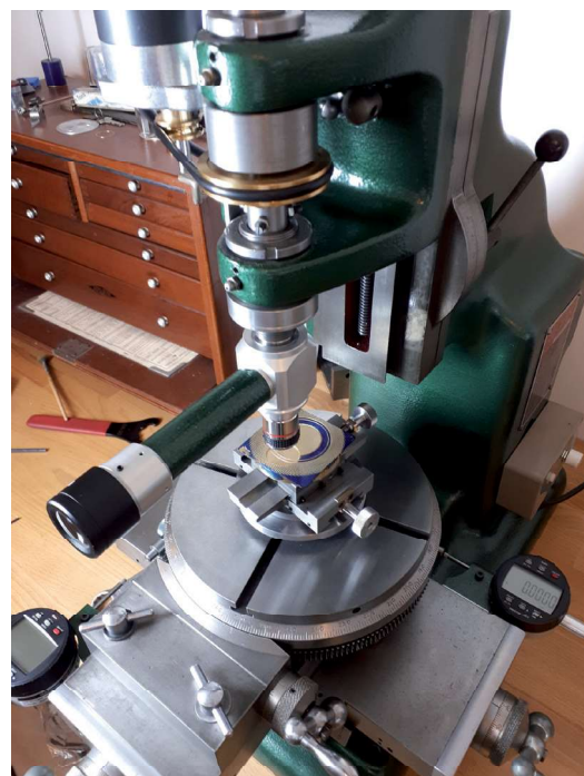
Fig.2 – Work holding compound table located in the jig borer
