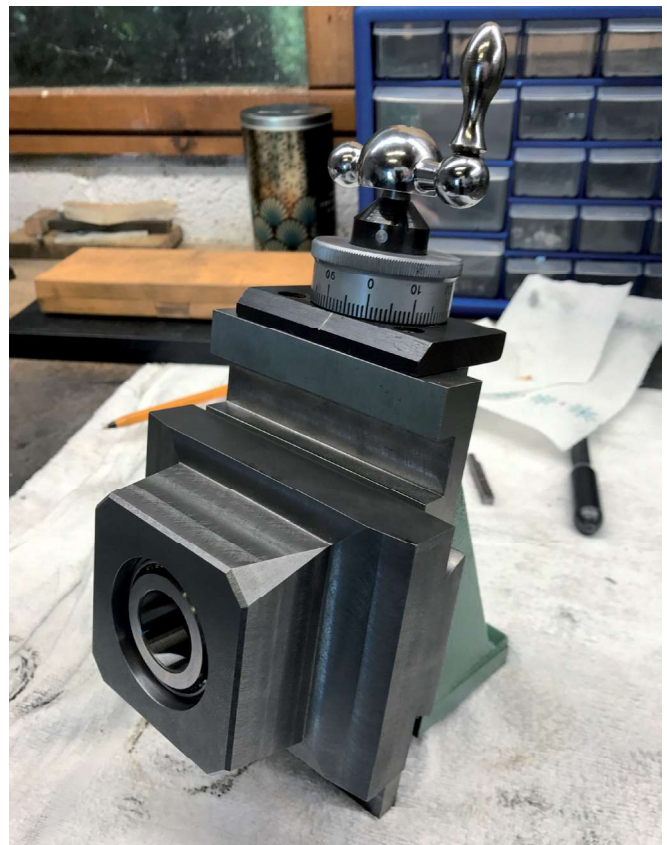
Fig. 5 – Assembly of part completed sliding head, showing tapered roller bearing
