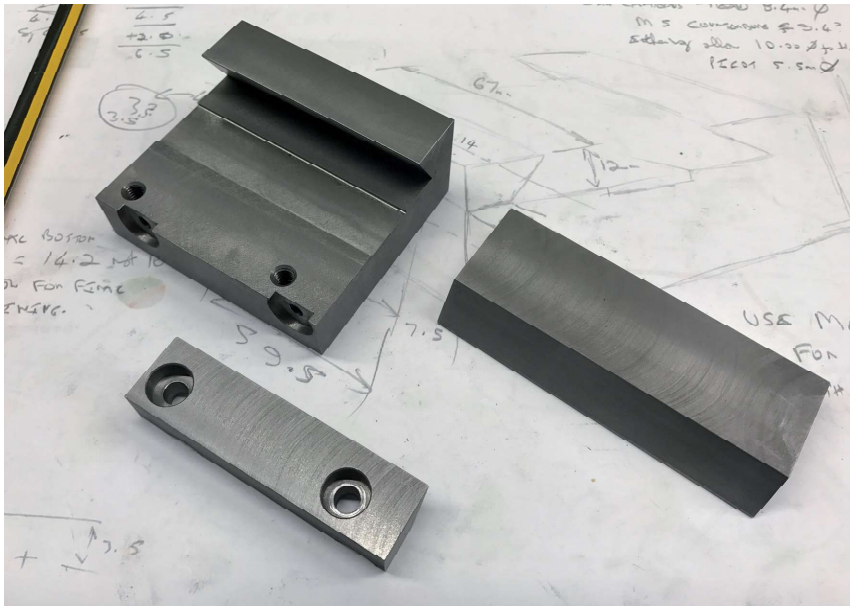
Fig. 8 Main tool slide components and initial working sketches
