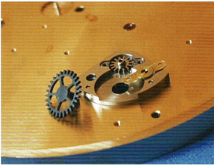
Figure 6. Part-finished components for the drive to the seconds hand.
