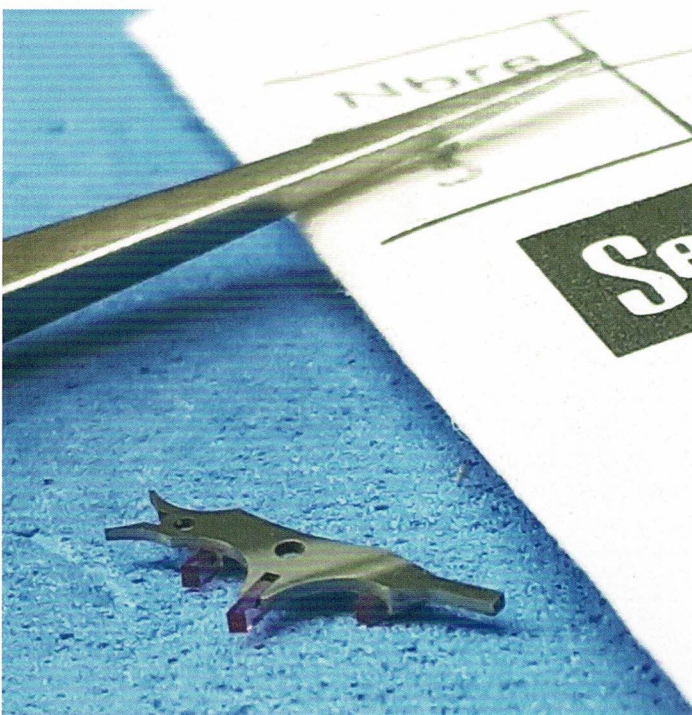
Figure 8. Lever for the Co-Axial Escapement.
